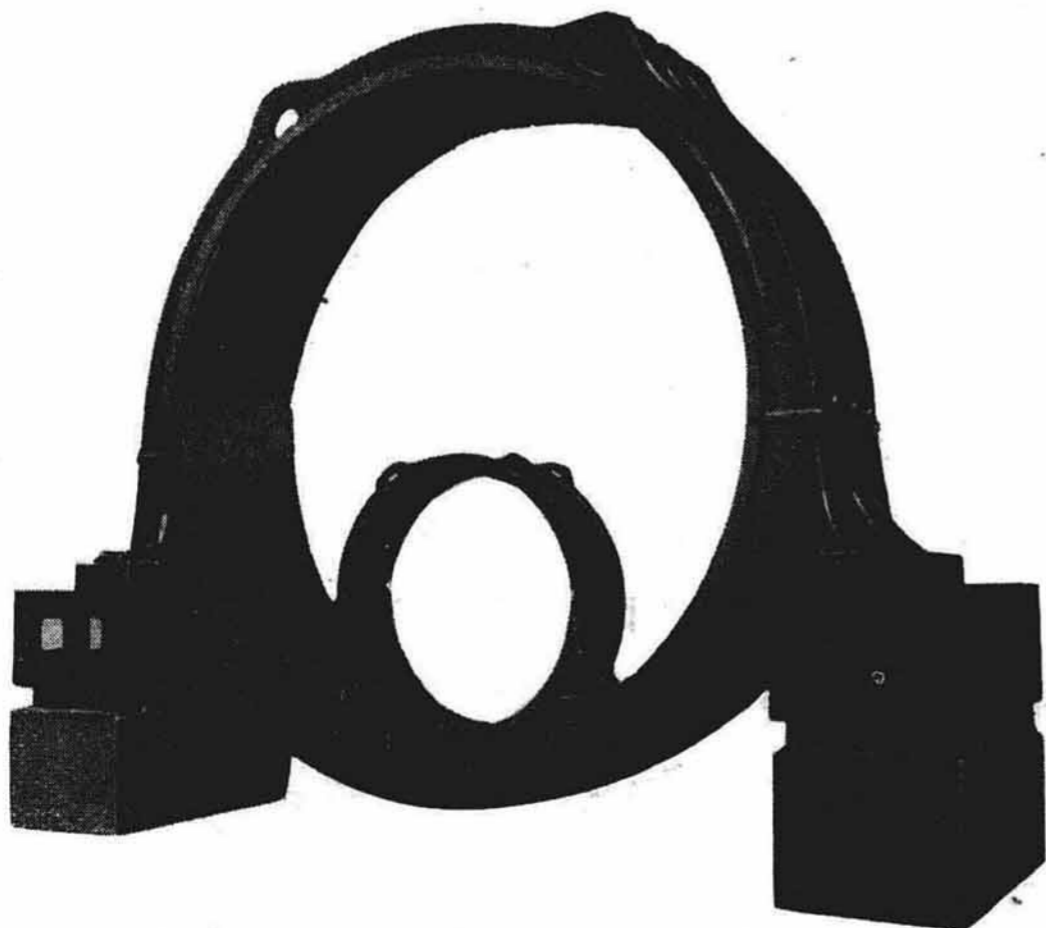
Yoke of 23,600 HP D.C. Mill Motor Compared with That of the 1,000 kW Standard Rotay Converter
