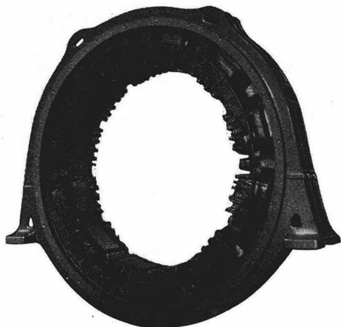
Stator of 2,000 kW D.C. Generator
