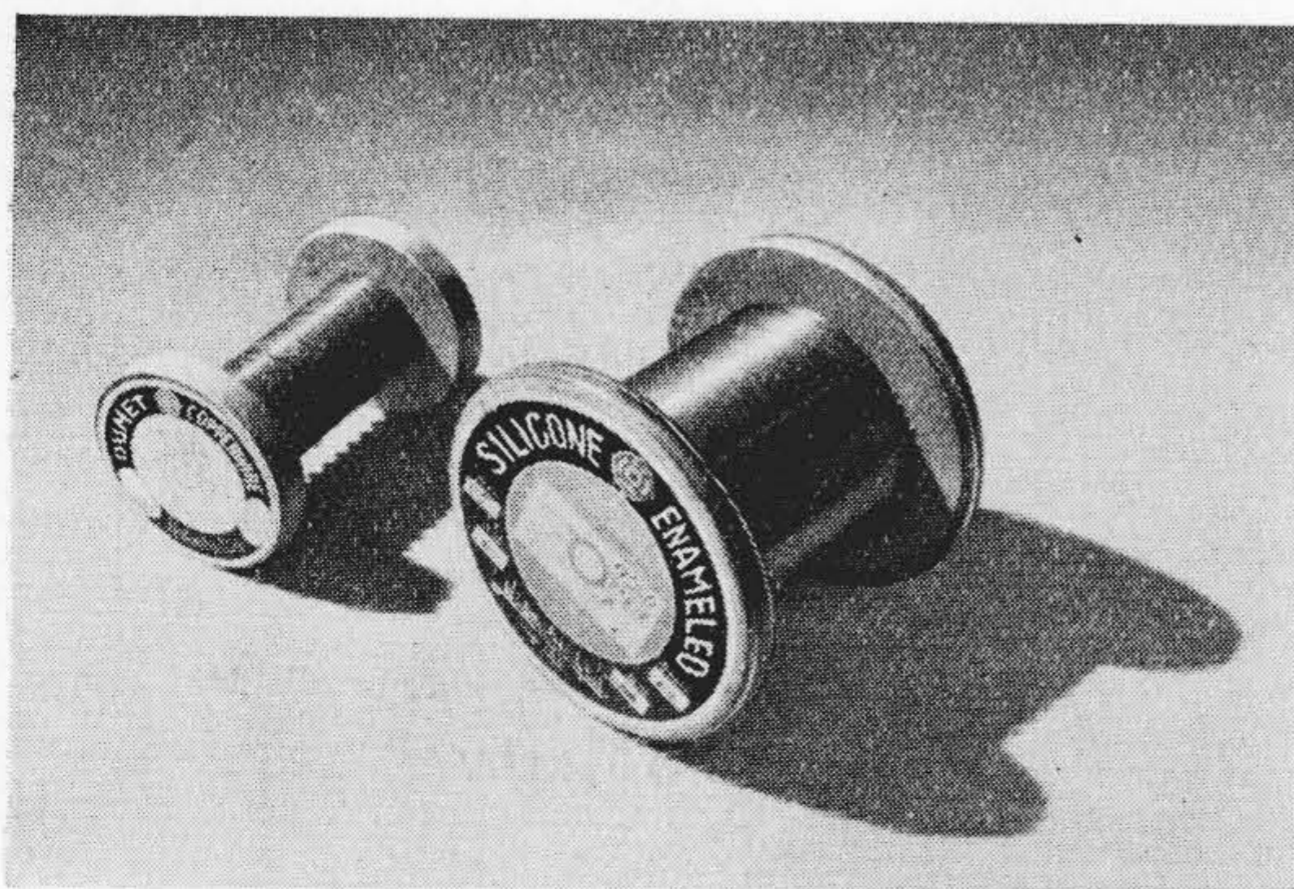
第 15 図 珪素樹脂ジメット線(向つて左) 珪素樹脂エナメル線(向つて右) Fig. 15. Silicon Resin Insulated Dumet Wire (Left) Silicon Resin Insulated Copper Wire (Right)
