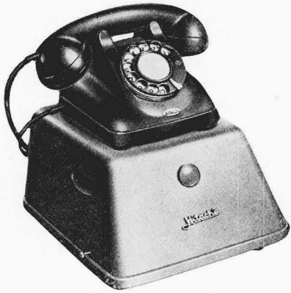
第3図 連接電話宅内装置外観 Fig. 3. Outside View of Subscriber Set of Party Line
