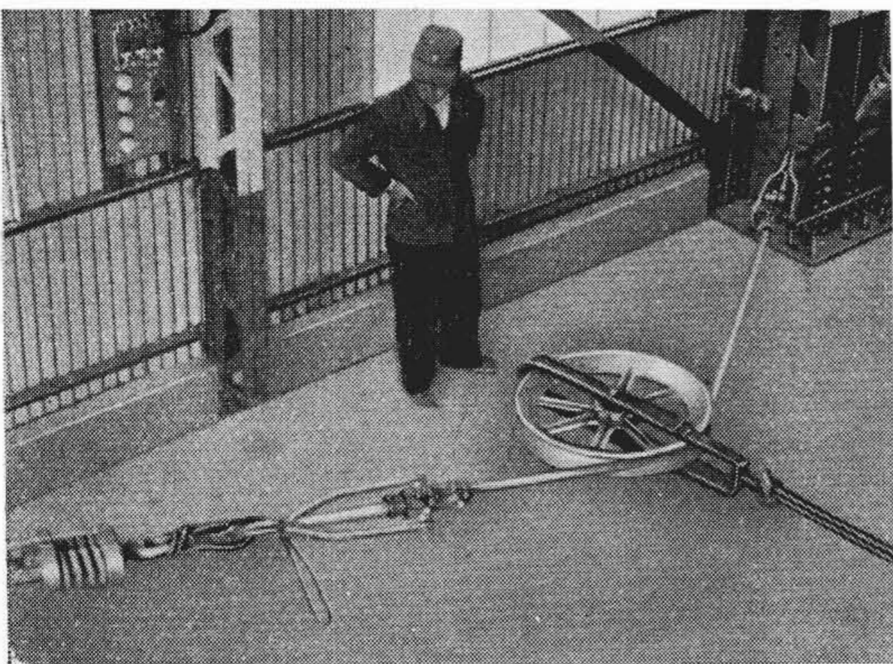
第7図 防蝕層の釣車通過による変化測定 Fig. 7. Measurement of Change of Protective Layer by Passing through Snatch Block
