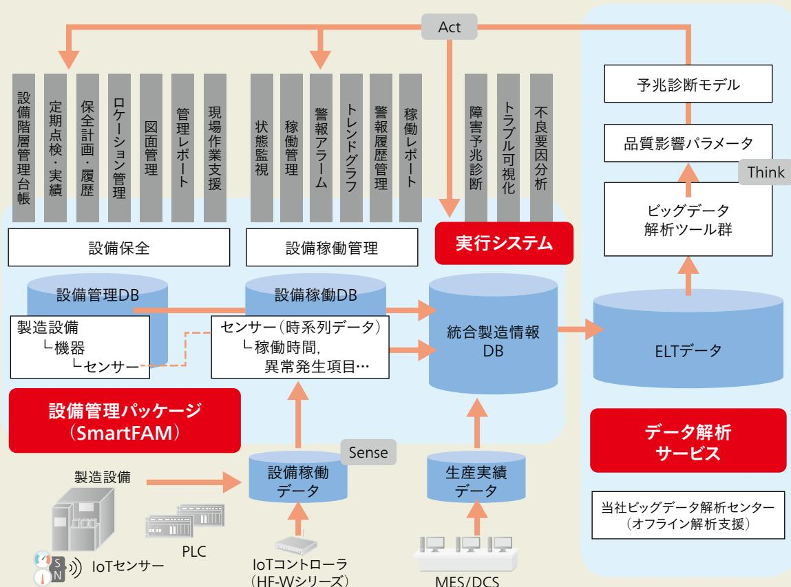
注：略語説明 DB(Database), PLC(Programmable Logic Controller), DCS(Distributed Control System), ETL(Extract, Transform, Load)
