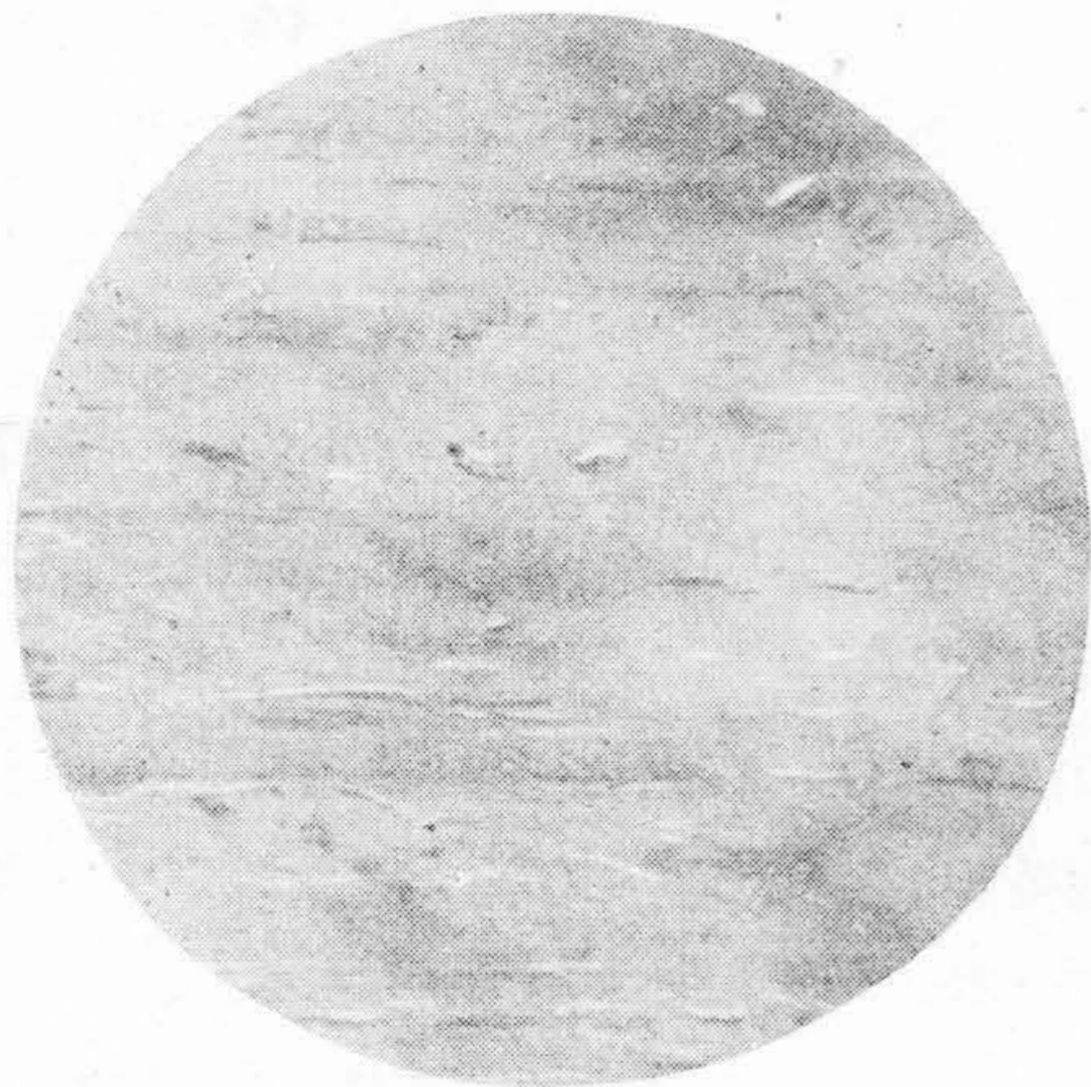
第 23 圖 精密研磨面 (加工流動層を示す) BK × 250 Fig. 23 Fine Ground Surface. (Working Flow Layer) BK × 250
