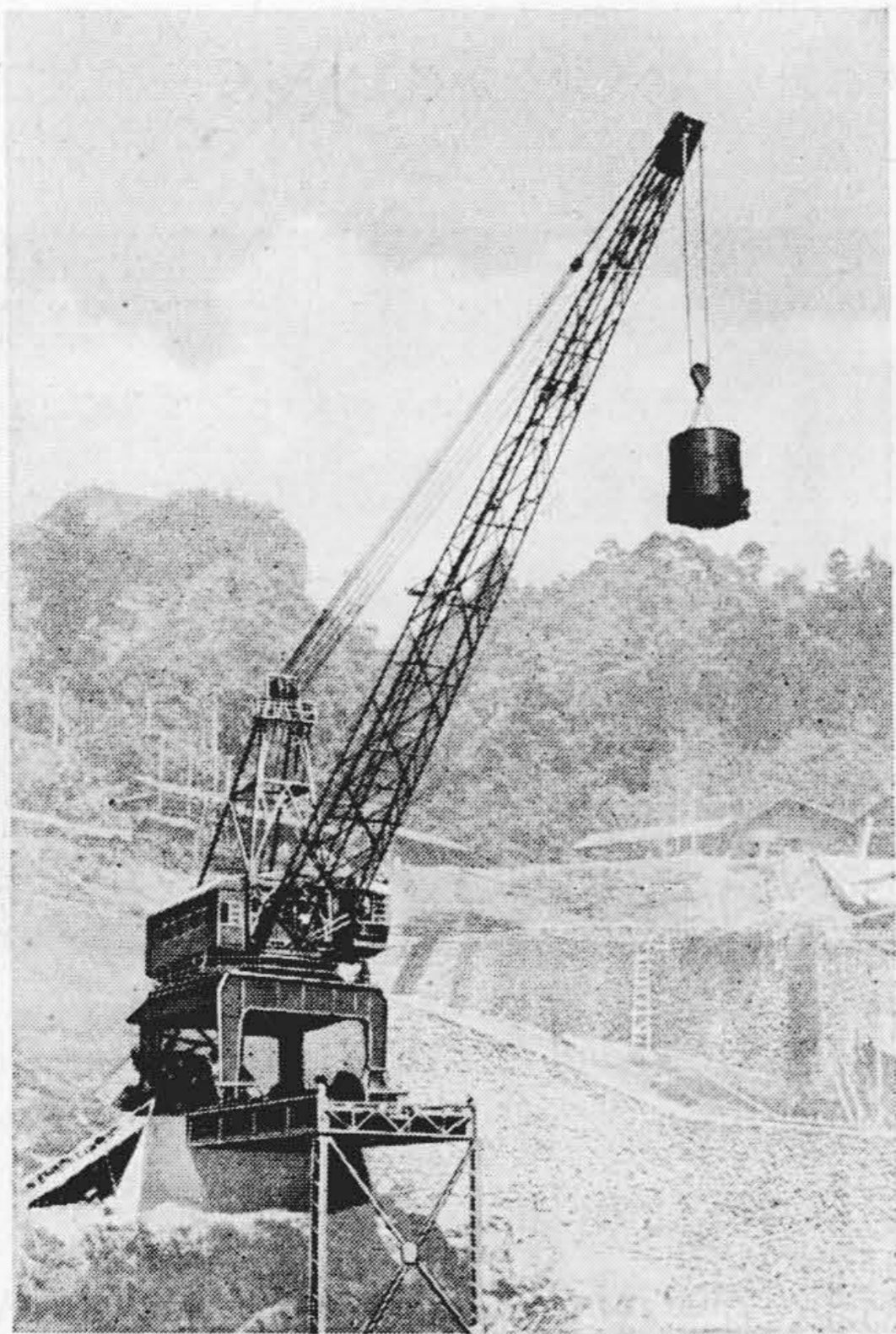
第 4 圖 9t 門型走行ジブ起重機 Fig. 4 9t High Pedestal Type Travelling Jib Crane with Concrete Bruket.
