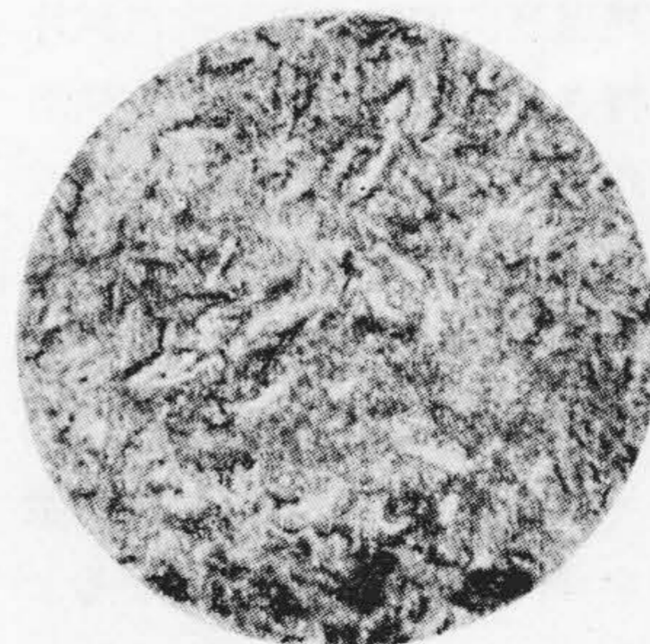
Fig. 18 Specimen No. 4 Austempered at 350°C for 70 Minutes and Quenched in Water (Austenitizing Temperature 920°C) Bainite.
