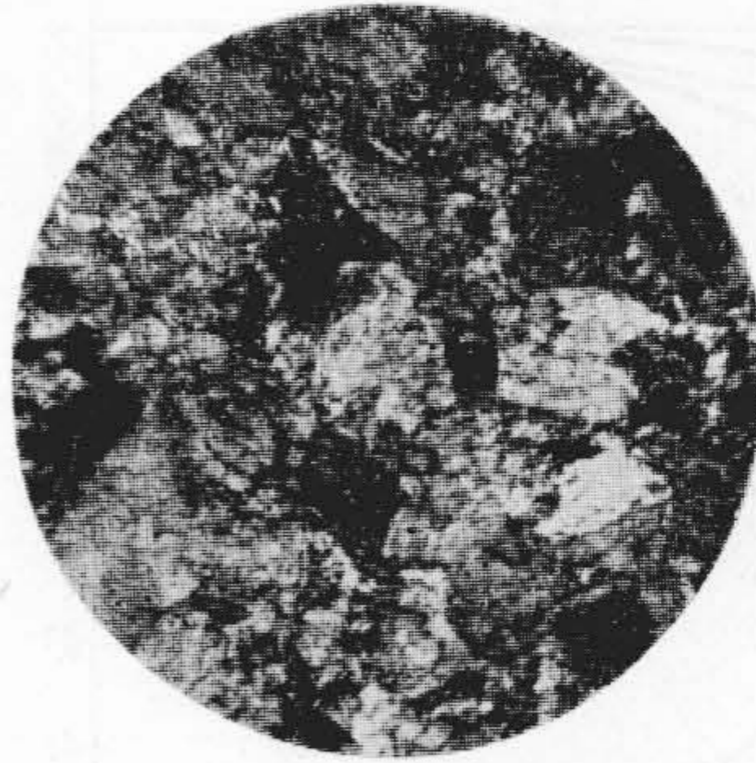
Fig. 10 Specimen No. 4 Austempered at 700°C for 5 Minutes and Quenched in Water (Austenitizing Temperature 920°C) Pearlite.
