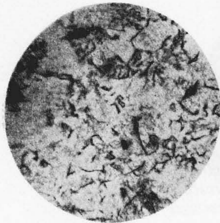
Fig. 13 Specimen No. 4 Austempered at 500°C for 30 Minutes and Quenched in Water (Austenitizing Temperature 920°C) Troostite+Martensite.
