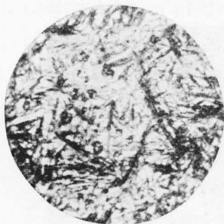
Fig. 12 No. 2-A Water Quenched structure at 1,150 °C (30 min) Normalized. ×400
