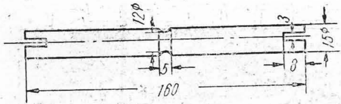
第 22 図 繰返し打撃試験片 Fig. 22. Dimensions of Test Pieces for Repeated Impact
