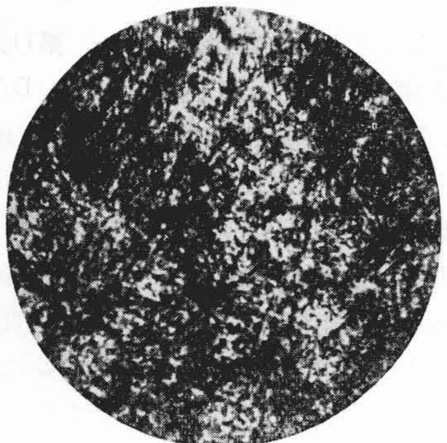
第15図 DAC 鋼の顕微鏡組織 (1,100°C 油焼入, 550°C 焼戻) ×400 Fig.15. Microstructure of DAC Die Steel (1,100°C Oil Quench, 550°C Temper)
