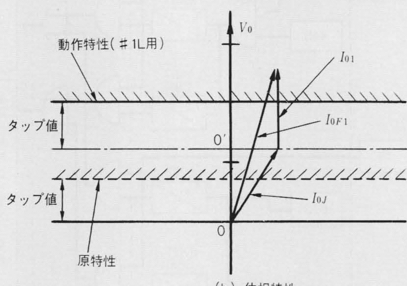
注：略語説明  $I_{0J}$ (零相循環電流),  $I_{01}, I_{02}$ (故障電流),  $I_{0F1}, I_{0F2}$ (零相電流), NGR(中性点接地抵抗器),  $V_0$ (零相電圧)
