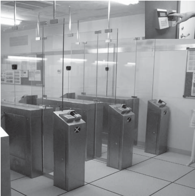
Fig. 2 | Finger Vein Biometric Technology for Security Management Finger vein biometric technology is a highly sophisticated personal identification system that balances security and convenience for assured authentication.
