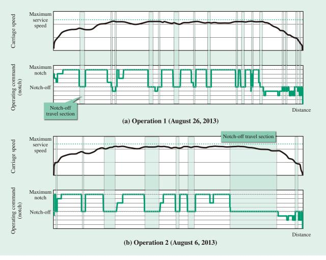
Fig. 4—Comparison of Carriage Speed Information and Operating Command Information in Section A. With travel under Operation 2 where the traction power consumption is small, travel was conducted under relatively long notch-off operations.
