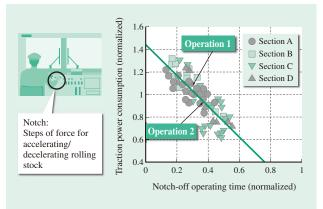
*Fig. 3—Relationship between Traction Power Consumption and Notch-off Operating Time.*
