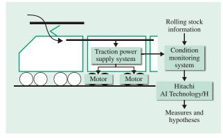
*Fig. 1—Example of Utilizing H for Rolling Stock Operating Information.*
