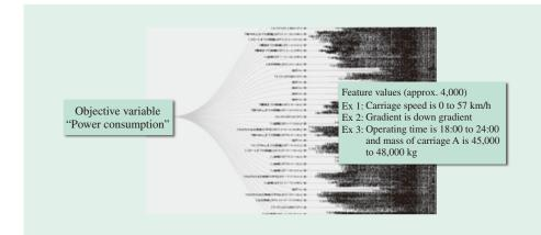
Fig. 2—Feature Values Generated by H. For H, approximately 4,000 feature values were automatically generated from the 12 explanatory variables. feature values. By analyzing the correlations between the objective variables and these automatically and comprehensively generated feature values, it is possible to gain knowledge and hypotheses that humans cannot process and that humans are not capable of noticing.
