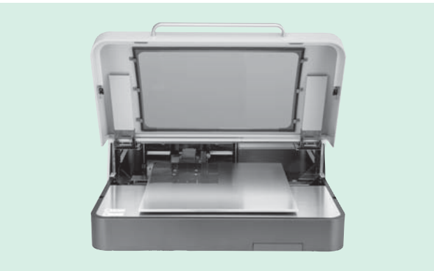
Fig. 2—FT150L with Sample Chamber Door Open. The large sample space provides ample room for large flexible samples.
