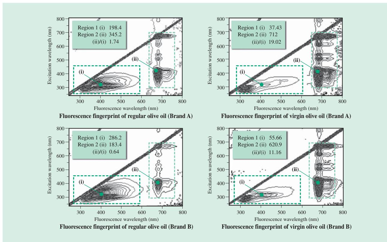
Fig. 8—Olive Oil Fluorescence Fingerprints.
