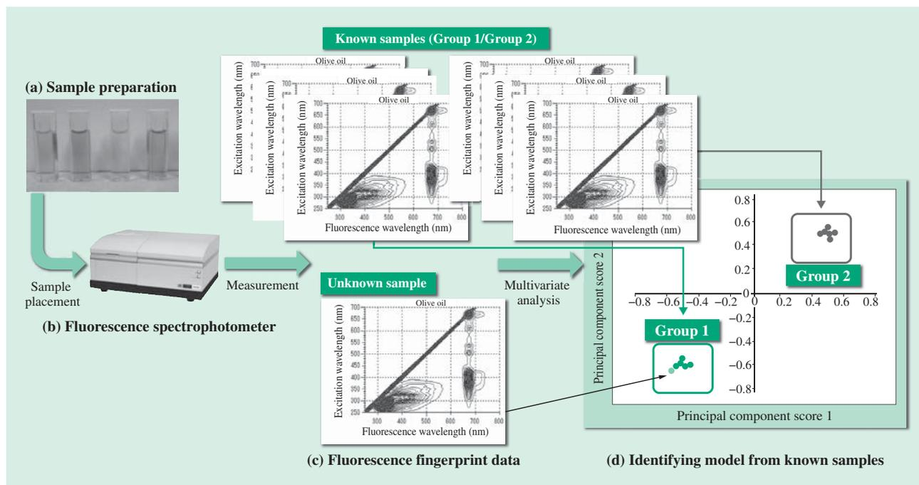
Fig. 2—Concept of Fluorescence Fingerprint Analysis Method.
