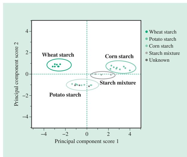
Fig. 7—Principal Component Analysis Results for Starch Fluorescence Fingerprints.
