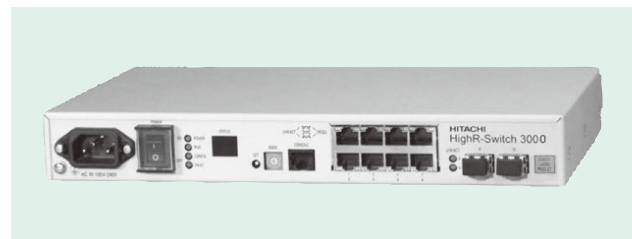
Fig. 6—Network Switch for Industrial Control Systems. It has been made more environmentally resistant, enabling installation in site equipment. In addition to providing typical network functions, it detects and automatically excludes unregistered communication.
