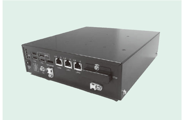
Fig. 4—Unauthorized Connection Detection Device. This device prevents the threat of cyber-attacks by detecting and automatically eliminating network connection attempts by unregistered devices.
