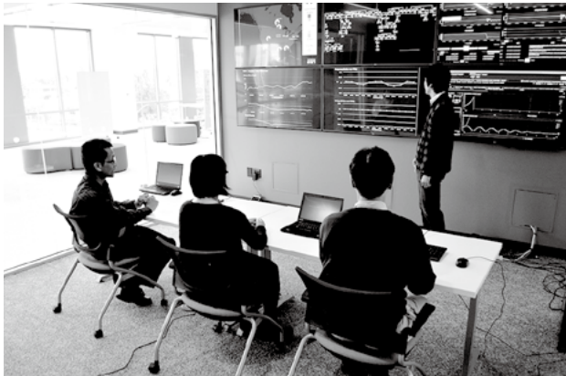
Fig. 3—Mini-control Room Demonstration. The mini-control room is used to demonstrate a DSS solution that combines online grid monitoring, event detection, high-speed similar case searches, and grid simulations.
