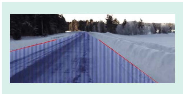
Fig. 4—Drivable Road Area Detection on Snow-covered Roads. The image shows the detection result when the road surface and shoulder are covered by snow. The red lines indicate the detected road edges. The area shaded by the blue lines indicates the detected drivable road area.
