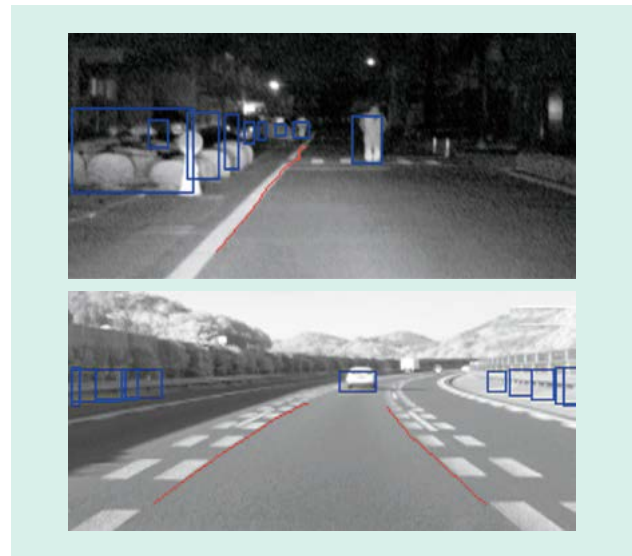
Fig. 3—Object Detection Using Stereo Cameras. The stereo cameras can detect vehicles, pedestrians, and any other objects. The blue rectangles in the image indicate object detection results, and the red lines indicate the white line detection results.
