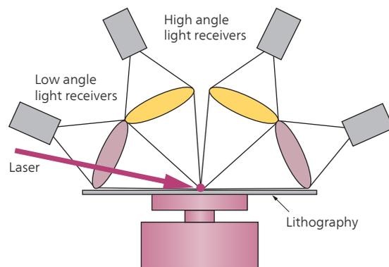
4 Wafer surface inspection system LS9300A (top) and structure of multi-detector light receiver (bottom)
