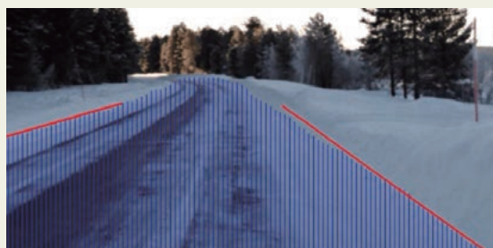
Figure 6 | Operation of Road Edge Detection (Detected Road Edge Shown in Red)
