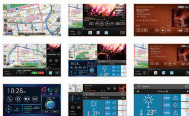
9 Quad view with capability for displaying a variety of functions and information on the same screen
