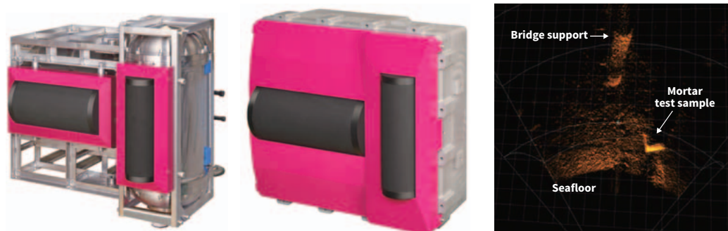
3 3D underwater acoustic video cameras [for deep ocean (left), and for shallow ocean (center)], and a video sample (right)
