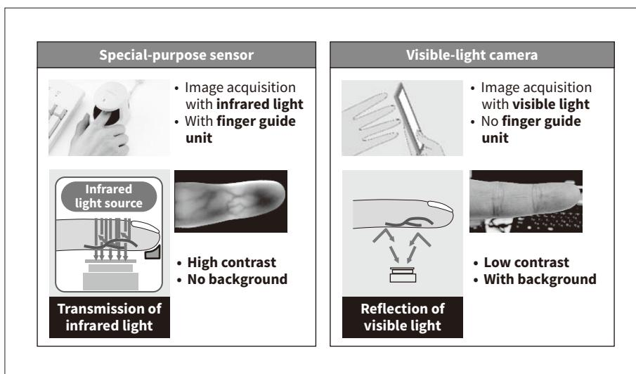
**Figure 2 — Differences between Imaging by Special-purpose Sensor and Visible-light Camera**
