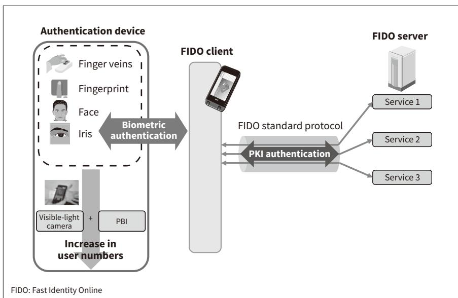
**Figure 5—Increase Service User Numbers by Integrating PBI-FIDO with Finger Vein Authentication Using Visible-light Cameras**
