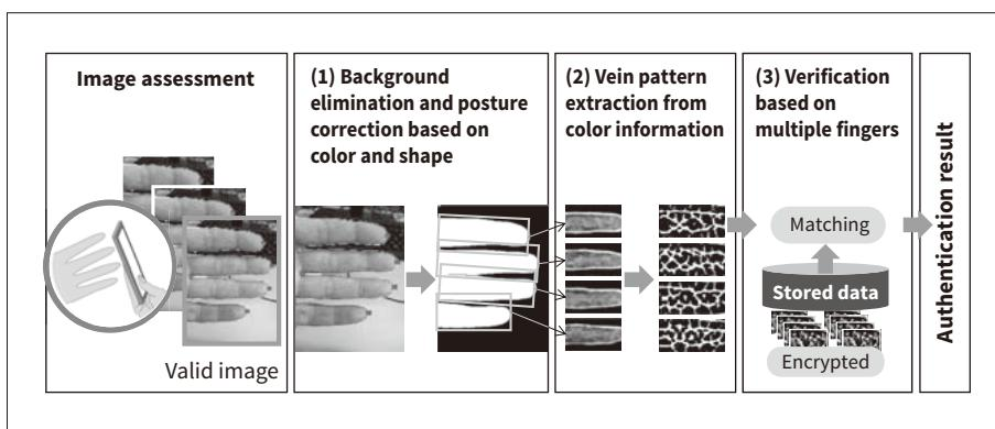
**Figure 3—Overview of Finger Vein Authentication Technology Using Visible-light Cameras**
