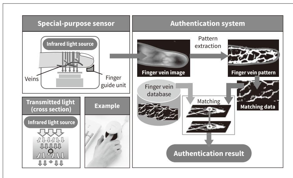
**Figure 1—Overview of Finger Vein Authentication Technology**
