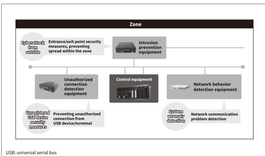
**Figure 4—Example of Integrated Security Monitoring for the Manufacturing Industry**
