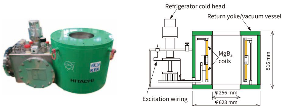
**3** Photograph and structure of MgB<sub>2</sub> superconducting magnet for klystrons
