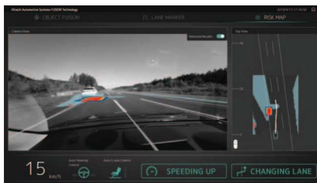
2 Risk prediction map generation (left), and autonomous driving using the risk prediction map to avoid a parked vehicle (right)
