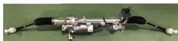
4 Fail operational belt drive EPS
