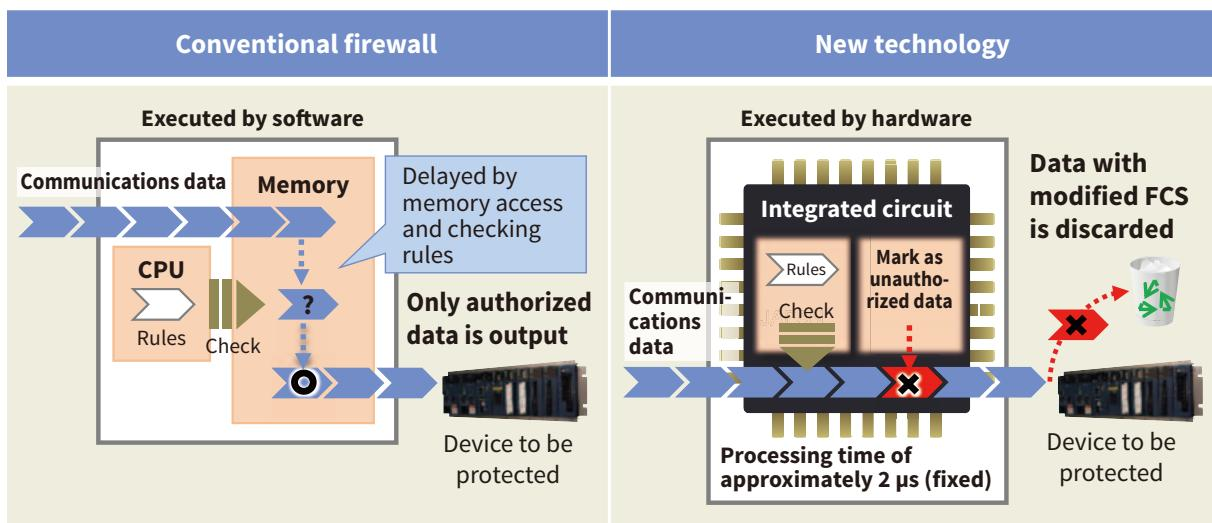
8 Real-time detection of unauthorized communications data (comparison with conventional technology)
