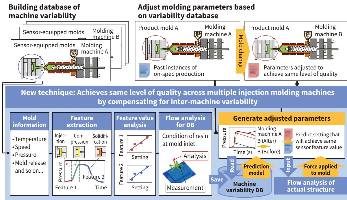
10 Overview of system for compensating for variability between different injection molding machines
