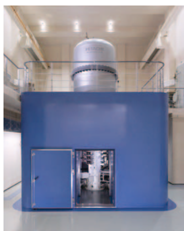
8 Atomic-resolution holography electron microscope (left) and image of electric potential distribution on gold nano-particle (right)
