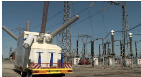
**23** Modular mobile substation for disaster recovery
