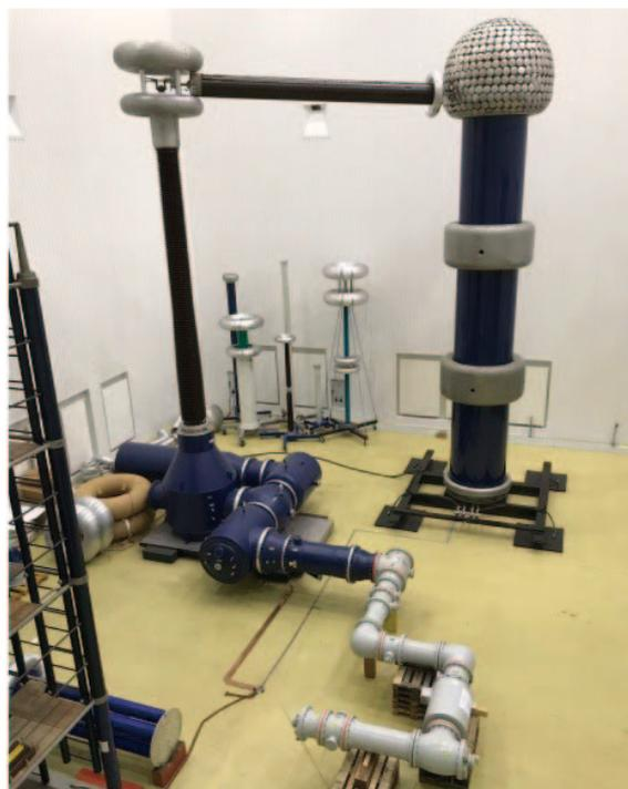
6 Dielectric type test of 420 kV passive elements in the high-voltage laboratory
