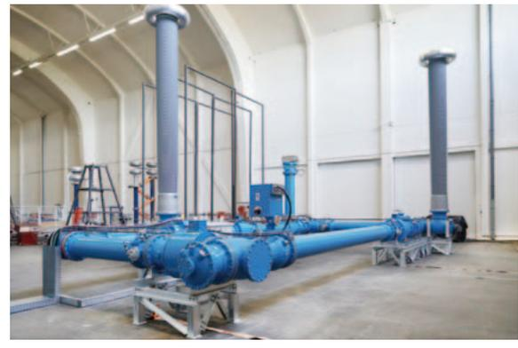
25 HVDC GIS prototype installation
