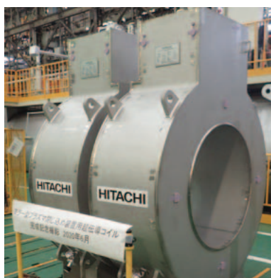
2 Two large conduction-cooled superconducting magnets after completion of manufacturing
