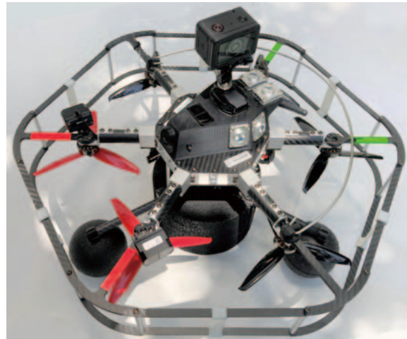
3 Sewer pipe inspection drone
