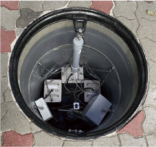
[11] Flow monitoring device installed in flow meter chamber (inner diameter 600 mm)
