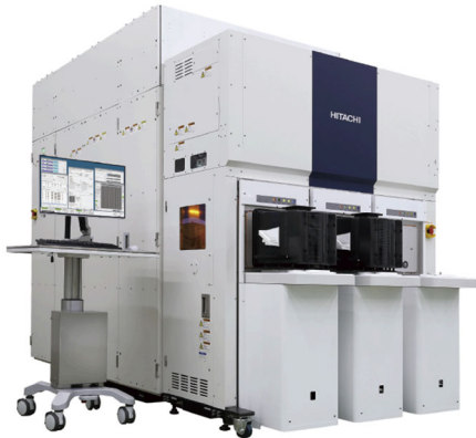
[02] GT2000 metrology system for next-generation EUV lithography
