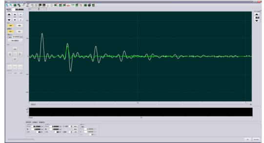
The screen shows the graphical user interface (GUI) for the waveform simulator. The white line shows the predicted waveform data for a multi-layer sample and the colored line highlights the echoes from the chip in the first layer.
