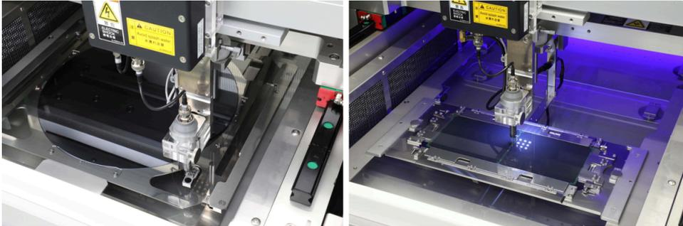
The photographs show a 300-mm wafer (left) and the FineSAT 7 water tank with a JEDEC-standard tray inserted (right).
