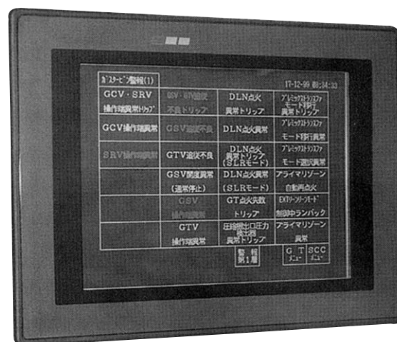
Fig. 8— Example of Warning Display on Flat Display. Aside from facilitating various types of displays, including operating data, warning windows, and individual warning factors, this display also has unconditional sequence master functions.
