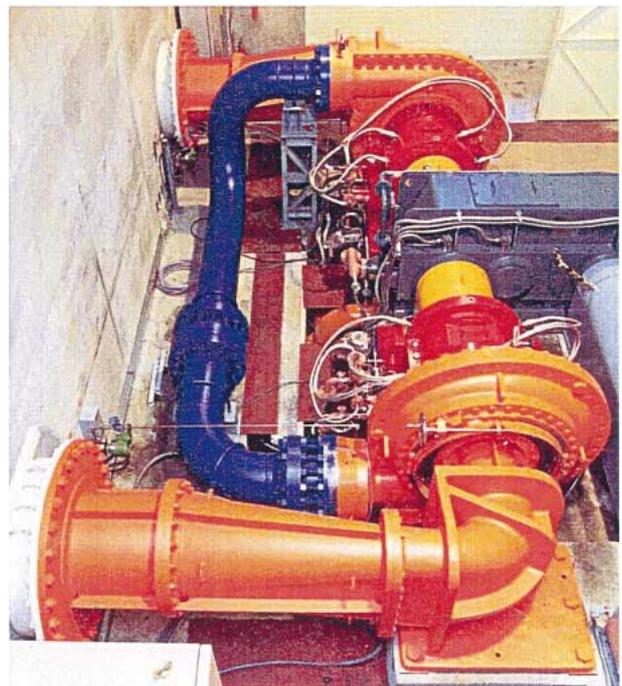
Fig. 4— Actual Head Model Test Equipment.
