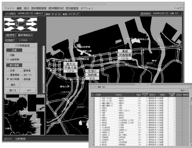
Fig. 4—Example of Control Room Monitor Display. By superimposing section travel times on the digital road map, information provision and management are integrated.
