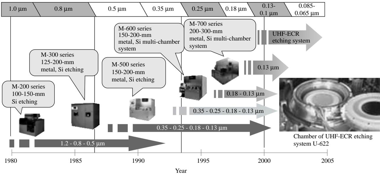
UHF-ECR: ultra high frequency electron cyclotron resonance
