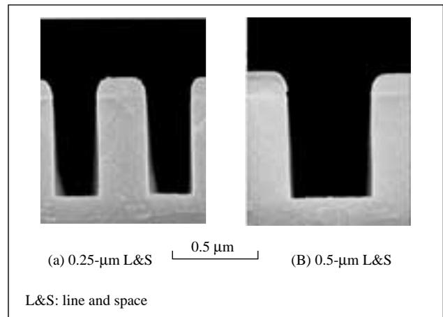
Fig. 8—Examples of Organic Film Etching. By controlling the antenna bias and wafer bias, excellent vertical profile, mask selectivity, and non residue etching are obtained.
