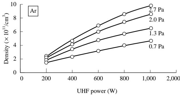
Fig. 3—Measured Plasma Density as a Function of UHF Power.
