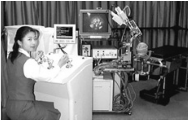
Fig. 2—Prototype of a HUMAN Manipulator System for Neurosurgery.
