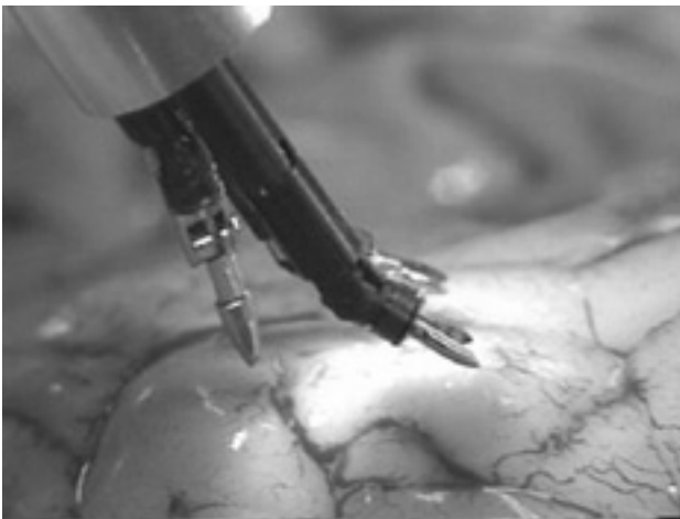
Fig. 3—Close-up of Insertion Section Tip. A magnified view of the tip of the HUMAN manipulator insertion section is shown; micro forceps are attached to the tips of three micro manipulators.
