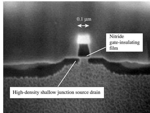
Fig. 4— Section Through a 0.1- $\mu\text{m}$  Transistor.
