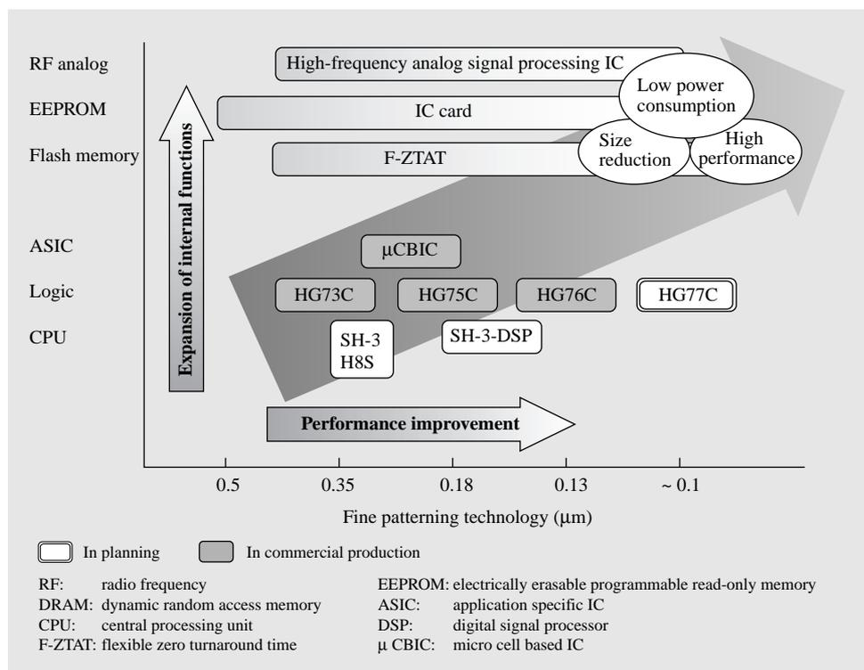
Fig. 1— Development of System LSI Chips by Hitachi. Hitachi has employed process technologies for embedding memories and analog devices as well as the most advanced CMOS (complementary MOS) transistors, in order to increase the performance and reduce the power consumption and sizes of systems-on-a-chip, centered on SuperH series RISC (reduced instruction set computer) devices.
