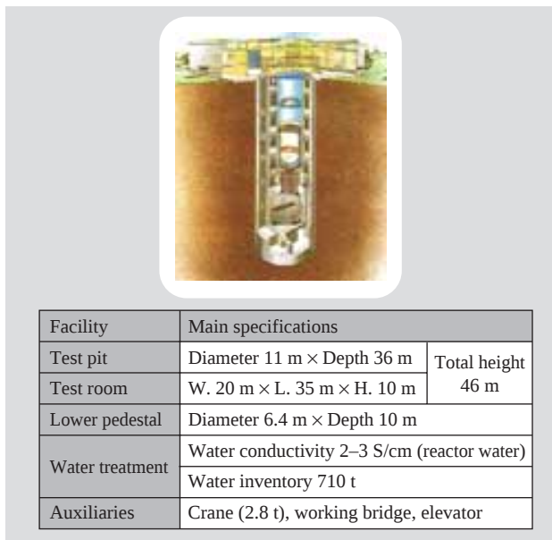
Fig. 9— BWR Maintenance Technology Center. The center is provided with full-scale facilities of a reactor pressure vessel and in-core structures, enabling the development of preventive-maintenance technology and processes for inspection and modification of major BWR equipment.
