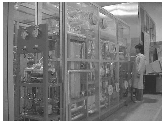
Fig. 5— This Fluorex Experimental Apparatus Is Used to Confirm the Method's Compatibility, Safety and Waste Generation.
