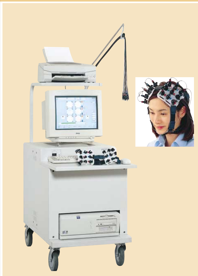
Optical-topography system Model ETG-100 is portable.
