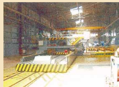
Inner view of the piping production factory (right) and a high-frequency induction heating pipe-bending machine for large bore piping (left)
