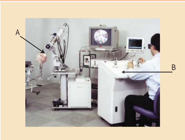
Prototype system supporting minimally invasive neurosurgery In a thin insertion probe, [A] three micro manipulators are bundled together; a surgeon is operating from an operating console [B]
