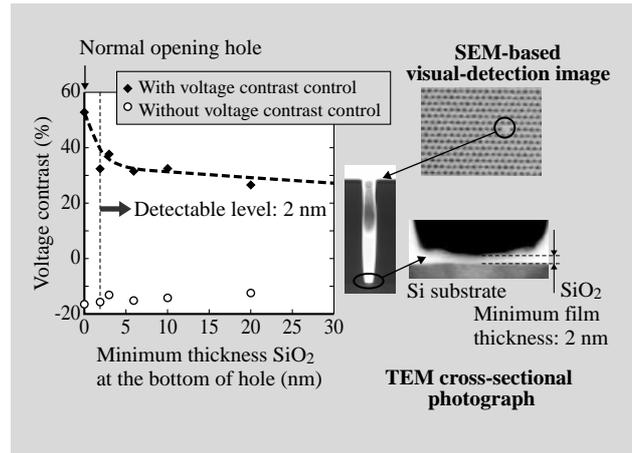
Fig. 6—Example of Residue Detected in Bottom of Contact Hole.
