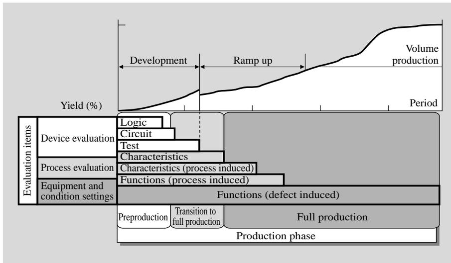
Fig. 3—Device Production Stage and Items for Evaluation.
