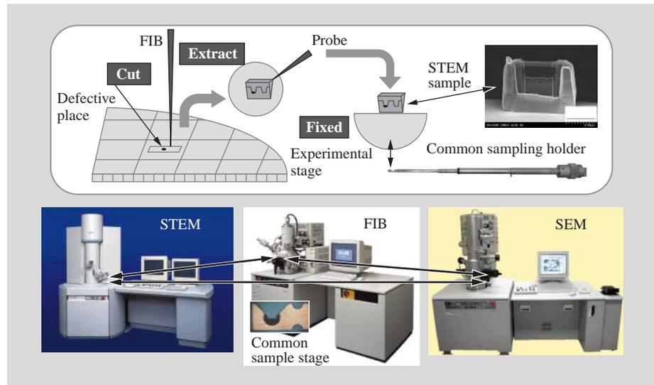
Fig. 10—Micro-sampling. The sample exposed to the FIB is attached to a probe and mounted on an experimental stage for observation. This permits high-resolution observation of the specific region in a short period of time.
