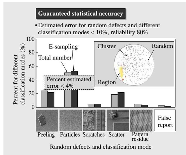
Fig. 9—Example of Data Showing Effectiveness of E-sampling. The error is less than 10% and reliability greater than 80% for 86 sampling points out of a total of 2,647 defects (actual result when all points are reviewed is 4%).
