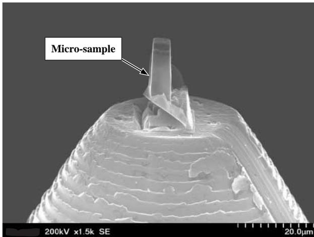
Fig. 4— $5\text{-}\mu\text{m}^2$  Pillar-shaped Micro-sample Prepared from DRAM (dynamic random access memory). By mounting the pillar sample on a corn shaped stub of the sample can be viewed and examined from all directions.
