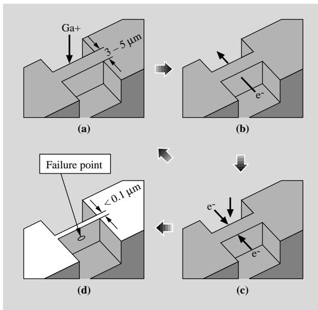
*Fig. 6—Locating Failure Point and Thinning Sample. A sample prepared a few microns thick (a) is mounted on the STEM and analyzed for defects (b) and (c). After determining the failure point, the sample is put back into the focused ion beam system and milled. By repeating the milling and the observations, the sample thickness is reduced to 0.1  $\mu\text{m}$  or less at the failure point (d).*
