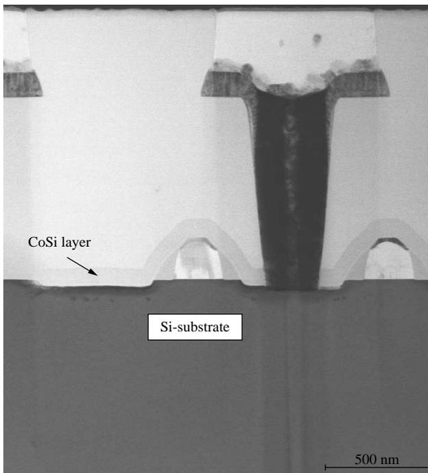
*Fig. 10—Low Magnification Sectional View of SH-Microprocessor (Transmission Image).*
