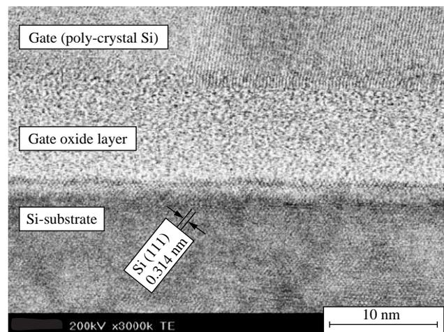
*Fig. 7—High-resolution STEM Image of Thin Si-device Gate Area Prepared by Using Semiconductor Evaluation System. The sample has been thinned to about 60 nm. A 0.314-nm crystal lattice spacing can be seen clearly at Si (111) plane of the Si-substrate and gate area.*
