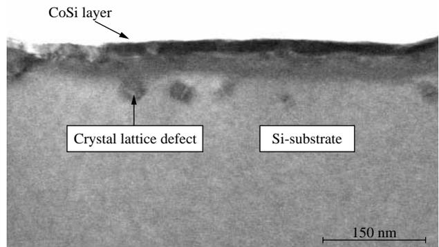
*Fig. 11—Sectional STEM Image of CoSi Diffusion Layer, SH-Microprocessor.*
