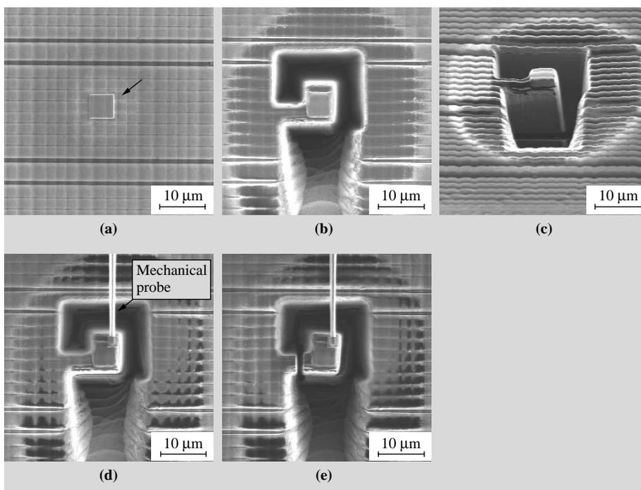
Fig. 3—Sequence of Micro-sample Preparation. The area of interest on a semiconductor device has been prepared. Scanning with a focused ion beam creates various sample shapes.
