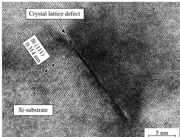
Fig. 12—Crystal Lattice Defect in Si-substrate below CoSi Diffusion Layer.
