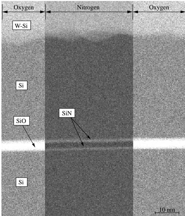
*Fig. 9—Insulation Layer Recorded by Using Real-time Light Element Mapping System.*
